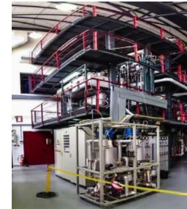
Pilot unit Circulating Fluidized Bed reactor (1 kg/h) CPERI/CERTH, Greece
